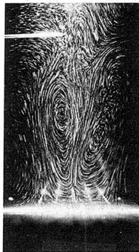
Fig. 13 Observed turbulence in the flow field, when the buoyant layer rises vertically and then splits. t_\infty = 3.1^\circ\text{C} , Q = 43.4 \text{ W/m} , and exposure time = 15 s. An impermeable surface is placed 1.4 cm below the energy source.
