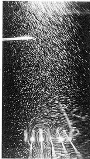
Fig. 11 Visualization of the flow at t_\infty = 2.3^\circ\text{C} , Q = 55.7 \text{ W/m} and exposure time = 20 s
